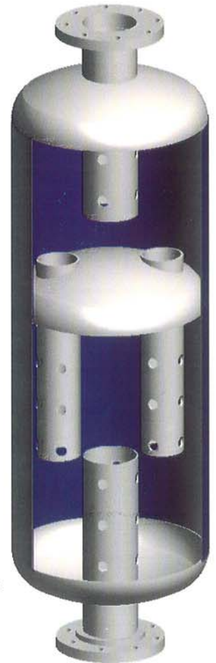
Figure 1.0 Typical Burgess-Manning reactive type silencer
