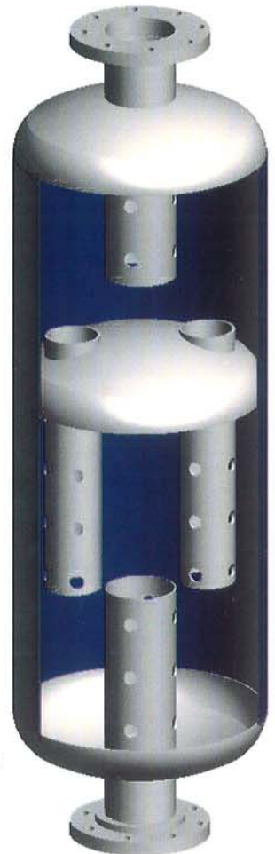
Figure 1.0 Typical Burgess-Manning reactive type silencer
